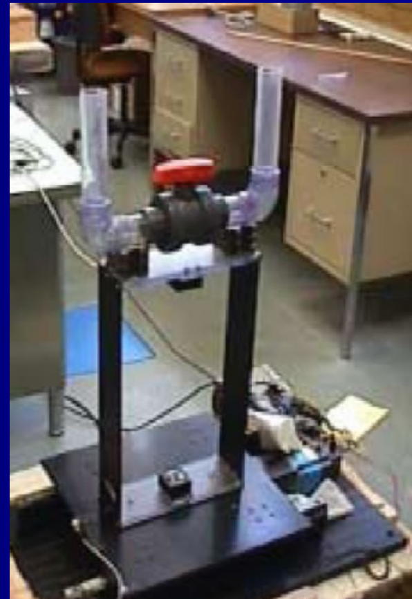
Figure 20 : Model of a TLCD on a vibrating table
