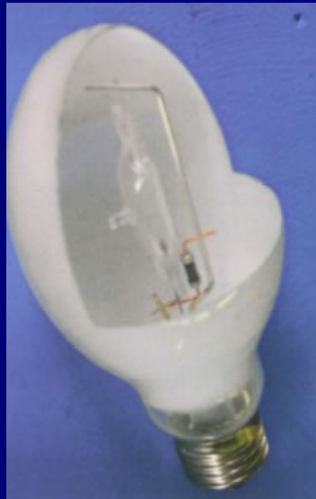
Figure 40 : detail of a ample broken by fatigue Due to pole mast vibration excited by wind
